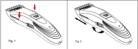
3. Adjust the trim length. Rotate the comb length ajustor and the comb will move up and down.(Fig. 2). There are 9 different comb position to adjust trim length from 3mm - 15mm.
