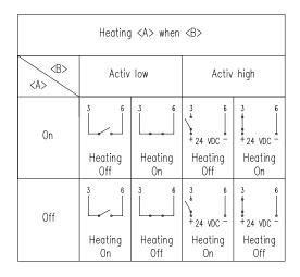
Different operating modes are available for controlling and monitoring the heating under moderate temperature conditions. The respective function can be set in the "u[sonic] Commander" configuration software.
