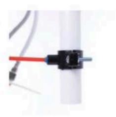
Push the red Tubing into the ¼ in. hole and secure with a Locking Clip.
