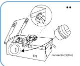
4 Run electrical wire from the power source through the mounting hole. Remove the right knockout and insert a connector(1/2 in) into it. Put the wire through the hole.
