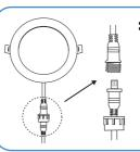
Connect the junction box and the light with the provided male/female connector. Do the connection with the arrow signs on the ends of cable aligned. Screw the cap to protect the connector.
