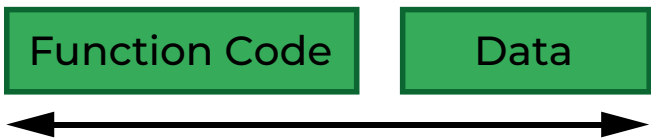
Fig.1 : MODBUS Protocol Data Unit
