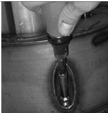
Tightening the glow plug using a dynamometric screwdriver (torque 0.65 Nm)
