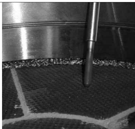
Glow plug correctly installed, in contact with the silicon carbide filter and in the centre of one of the 4/6 segments
