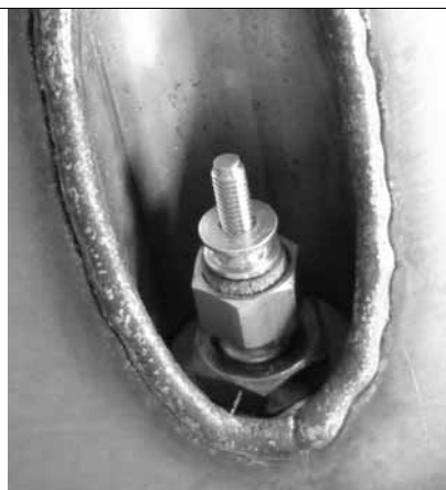
Glow plug installed, secured with M10x1.25 locknut (torque 25 Nm)
