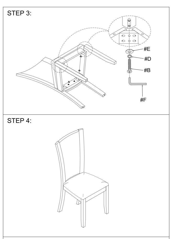
Tighten all screws until completely asembled.
