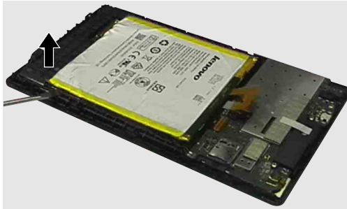
Figure 4. Removal steps of battery pack (continued) Insert a flat blade to detach the battery pack.
