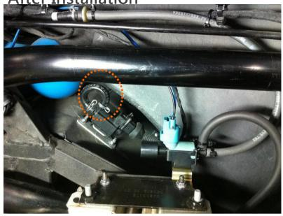
CONNECT THE STOCK "IN" AND "OUT "SOLENOID VALVE TOGETHER WITH CALBE LINES. SEE THE IMAGE ON YOUR LEFT HAND SIDE.
