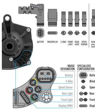
BLIND PLUG plug without pins to seal unused motor ports
