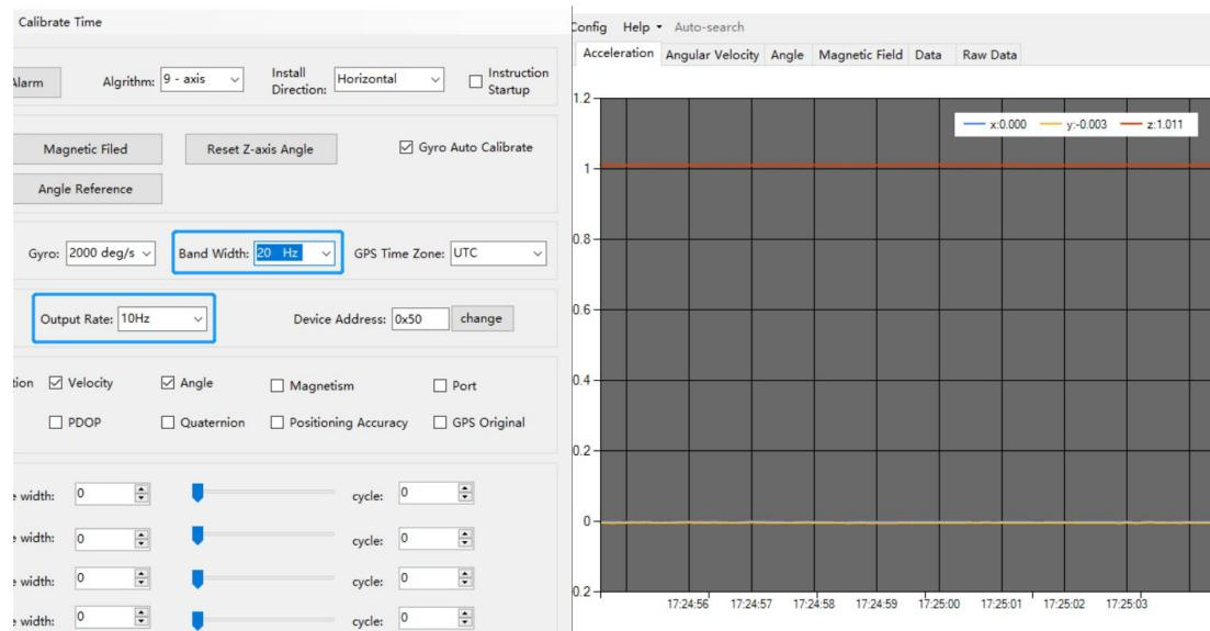
Bandwidth as 256Hz, Output rate as 10Hz. The waveform will show more fluctuation.
