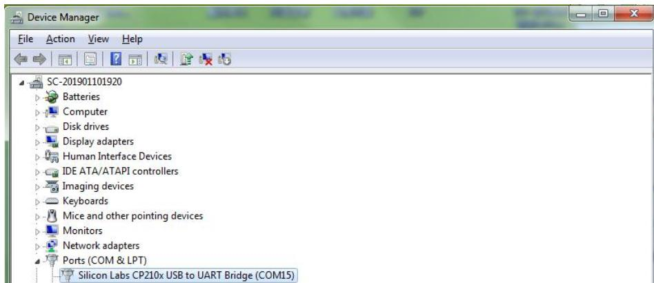
**Step 2.** Insert the converter to computer and confirm the "com port" in device manager
