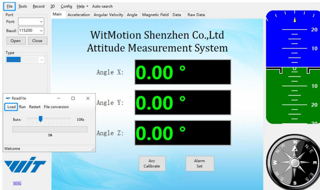
Step 3: Choose the original path of software installation and load the Bin file
