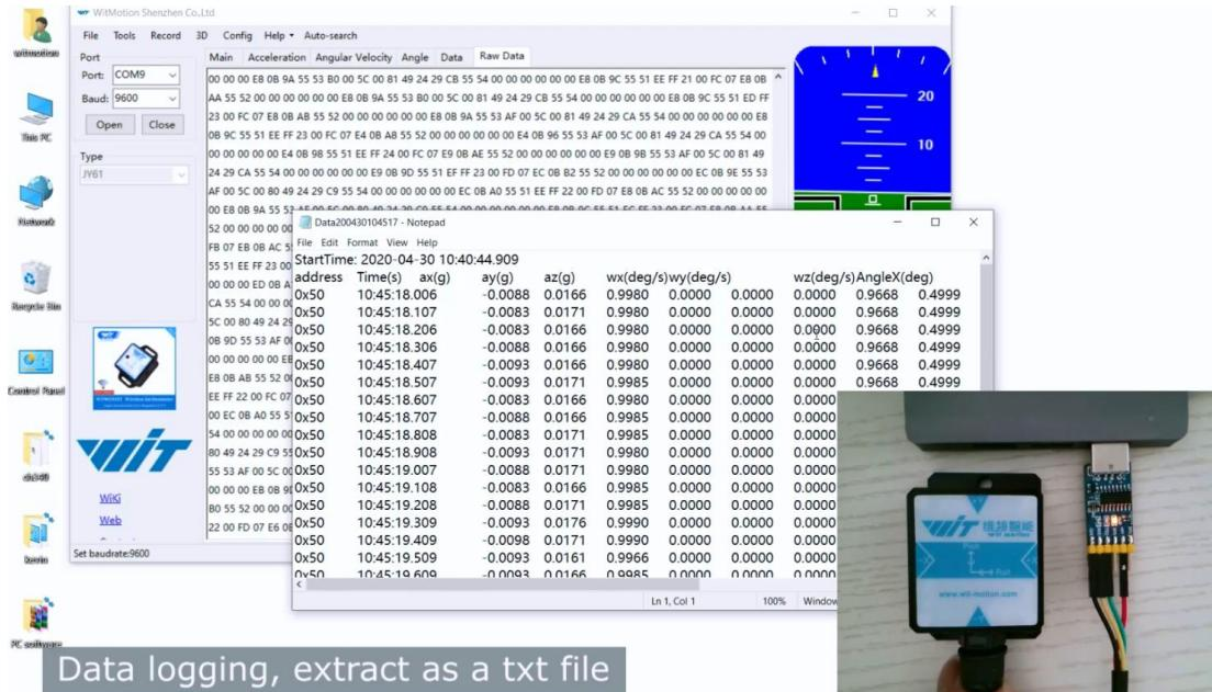
Notice: If there is repeated "TIME" of data, that's caused by low-resolution of the Windows system's time. The changes in other data is correct.
