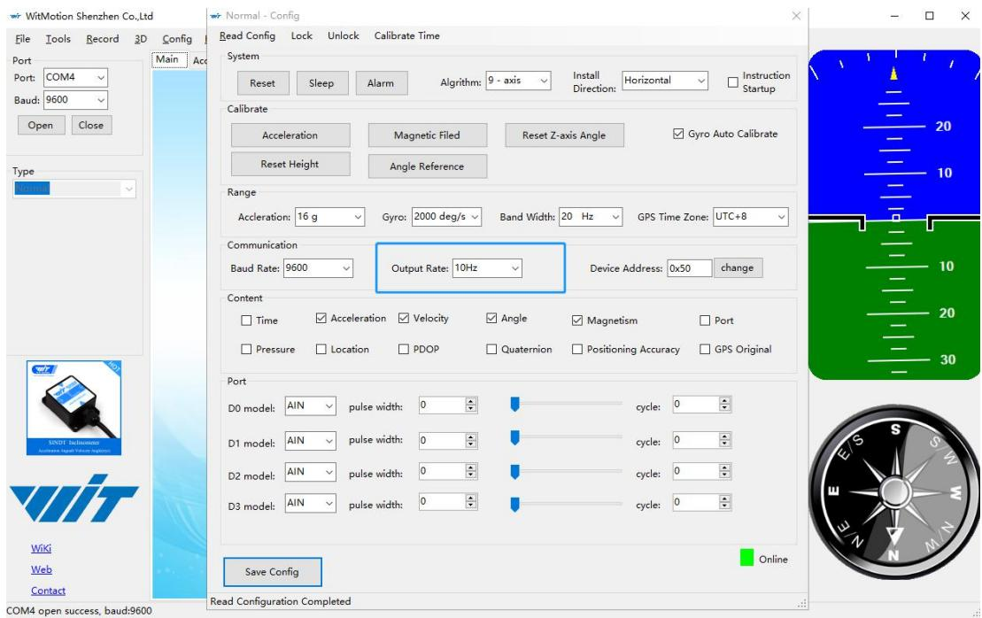
The default return rate of the module is 10Hz, the highest return rate supports 200Hz.
