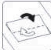
Remove the parts from the frame with a rotating motion along the groove formed by the bits you just cut.
