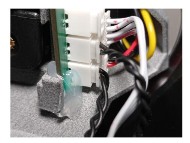
4) This picture shows the connector for button #2 with one of the pins showing. This connector is faulty. The pin must be re-inserted fully for the button to work correctly.
