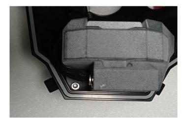
2) Remove the screw so it can't fall into one of the domes, then lift the tray and place it on the inside of the housing. This will expose the 4-pin XH-type LED connector and two 2-pin XH-type button connectors.
