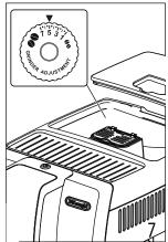
The coffee grinder is set by default to prepare coffee correctly and should not require regulating initially.
