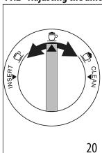
Turn the froth adjustment dial (D1) (fig. 20) to adjust the amount of froth on the milk delivered while making cappuccinos and milk-based coffees.
