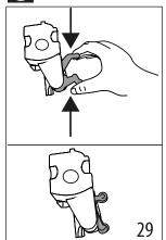
If the infuser is difficult to insert, before insertion, adapt it to the right size by pressing the two levers (fig. 29).
