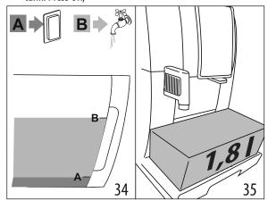
"Pour descaler and water into tank": Pour the descaler into the tank up to level A (corresponding to a 61 fl oz /100 ml
