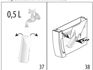
Extract the tank (A17) from the appliance and fill with water;
