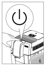
To turn the appliance on, press the button (A7) (fig. 6). The message "Heating Please wait" appears on the display (B1).
