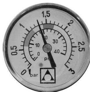
1,3 kg/cm 2 - 18,5 PSI: This pressure indicates that it is necessary to "BACKWASH".
