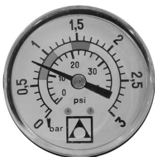
0,8 kg/cm 2 - 11,4 PSI: Normal pressure at the beginning of a filtering cycle.
