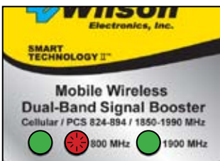
Red light on frequency indicator
