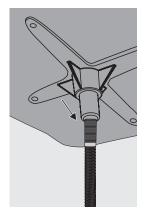
Put the seat onto the threaded rod.
