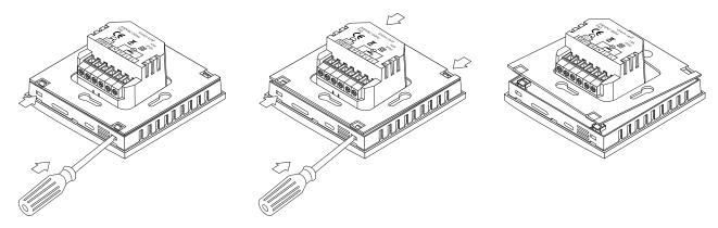
Step 3: Screw the metallic support frame to the in-wall box
