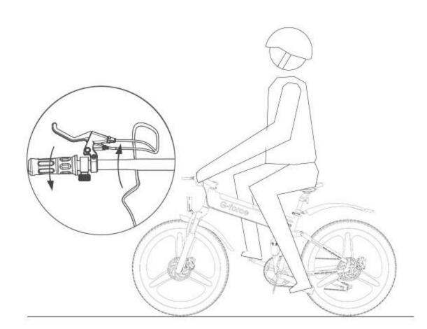
4. After releasing the accelerator or active brake, the motor will suspend to provide power
