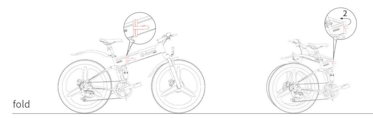
Make sure the electric car is turned off. To fold, unlock the folding mechanism, 1. Open the folding buckle of the riser before bending the handlebar; 2. Open the seat tube lock; remove it from the buckle, erect the handlebars and lock the folding structure
