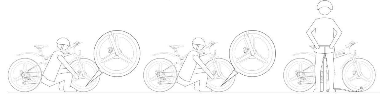
If the tire leaks, remove the screw cap from the valve, and then connect the extended nozzle adapter to the valve to inflate.
