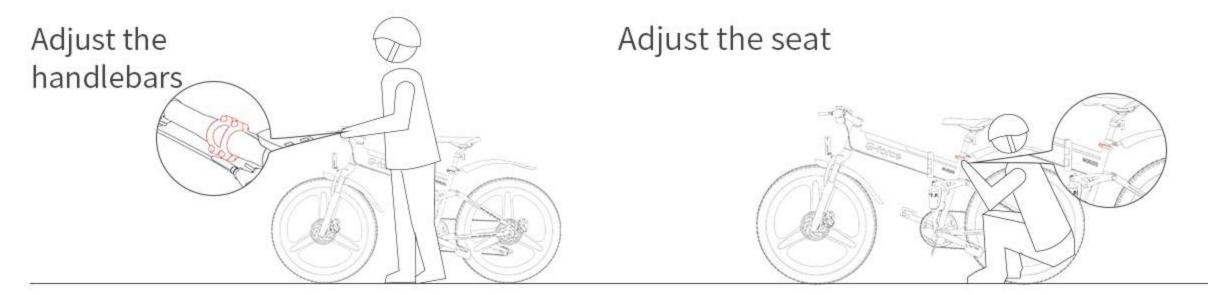
If the bicycle handlebar and handlebar stem swing during riding, use an M5 hex wrench to tighten the screws on the folding device.
