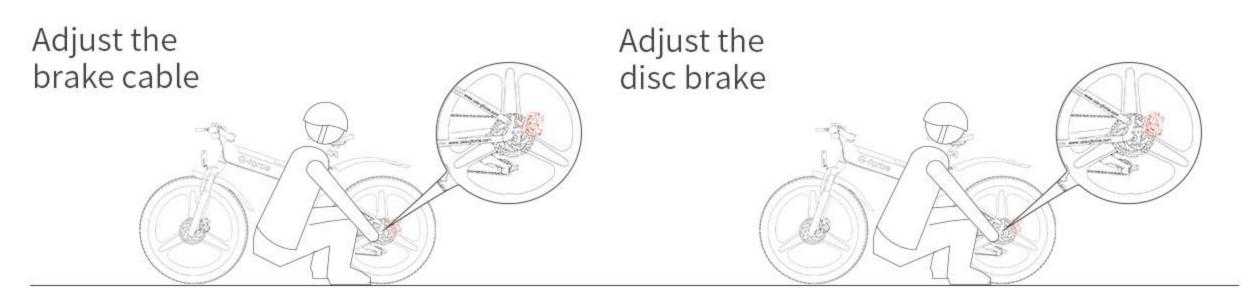
If the brake is too tight, use a hex wrench to loosen the screw on the caliper, then send the brake cable back slightly to shorten the bare length, and then tighten the screw. If the brake is too loose, loosen the screw, then gently pull out the brake cable to extend the bare length, and then tighten the screw.
