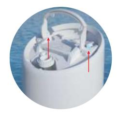
Lift the handle and move the housing locks to remove the TREAT housing
