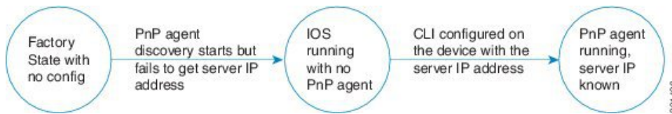
Figure 28: State Diagram for PnP Trigger with CLI Configured PnP Profile
