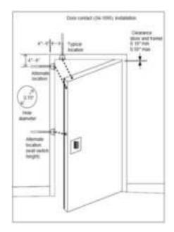
The image above shows the recommended mounting for the 04-1095 flush mount S241 switch on a standard door. This also applies to a sliding window or balcony door with a frame that can accommodate the 04-1095 flush mount S241 switch. However, in most cases, the 04-1097 surface mount S241W would be used, as described below.
