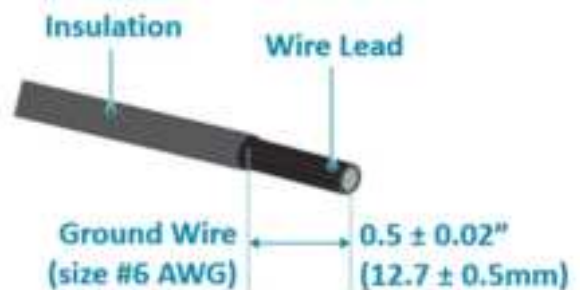
6-AWG green-and-yellow wire for grounding
