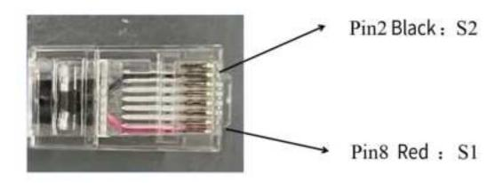
• RJ45 port definition for matching single-phase off-grid inverters
