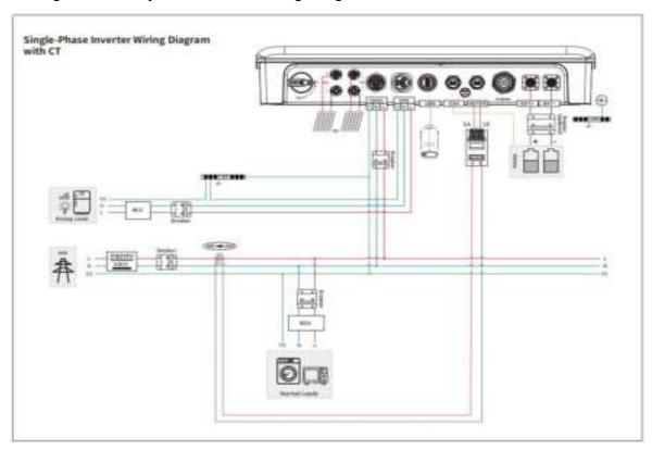
• Single-Phase Hybrid Inverter Wiring Diagram with CT (Only for Australia and New Zealand installation site).
