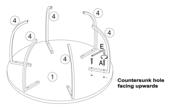
Tighten screws only after all parts have been property assembled.
