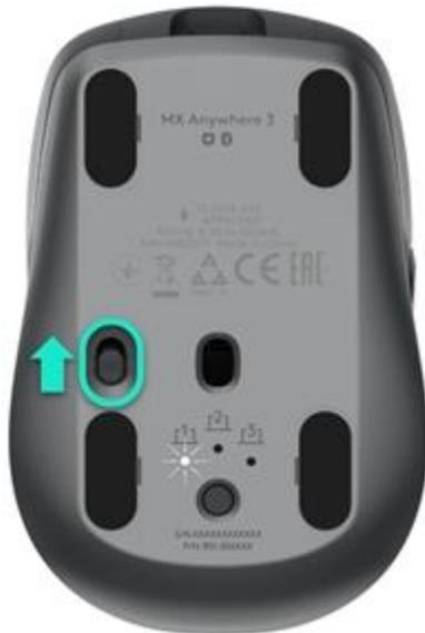
The number 1 LED on the bottom of the mouse should be blinking fast.
