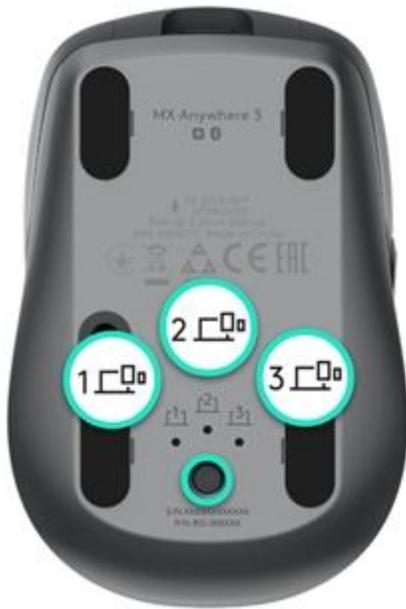
1. A short press on the Easy-Switch button will let you switch channels (from one computer to another). Select the channel you want and go to the next step.
