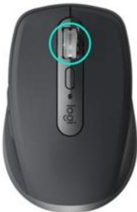
The speed-adaptive scroll wheel shifts between two scrolling modes automatically. As you scroll faster, it will automatically shift from line-by-line scrolling to free-spinning.
