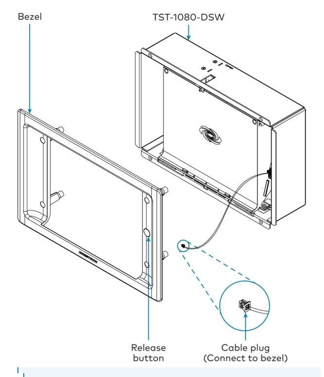
**NOTE:** If the bezel must be removed for any reason, disconnect this cable carefully prior to removal.
