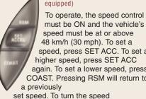
48 km/h (30 mph). To set a speed, press SET ACC. To set a higher speed, press SET ACC again. To set a lower speed, press COAST. Pressing RSM will return to
