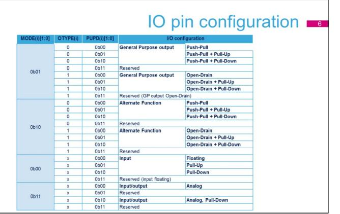
The configuration of any IO pin is achieved through 4 registers: GPIOx\_MODER, GPIOx\_OTYPER, GPIOx\_OSPEEDR, GPIOx\_PUPDR.
