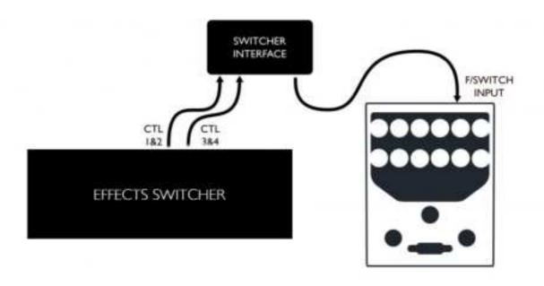
**NOTE:** Remote switching of the bypass state and active channel can only be achieved with the Switcher Interface. The interface converts latching control formats to a short momentary pulse. In the unlikely
