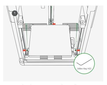
Remove the three screws with an Allen Key H2 to unlock the hot bed.
