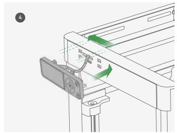
Inset the screen back to the slot on the printer, then lock it by pushing it to the left.
