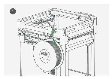
Insert filament into the PTFE Tube. Keep pushing the filament until it can not move forward.
