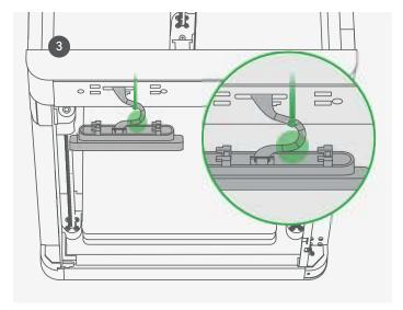
Attention: Bend the LCD cable towards the opening on the back of the screen as pictured.
