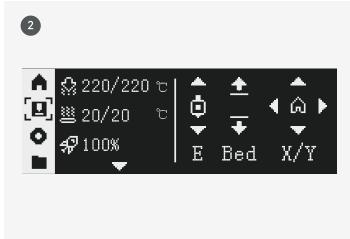
Select " ■ "-" ♀ ", and heat the nozzle to the recommended temperature for the filament.
