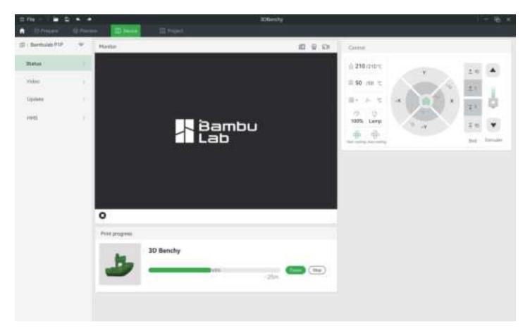
During printing, you can remotely monitor your print, or pause/stop printing on the "Device" interface.
