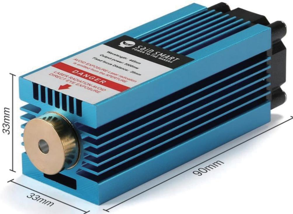
A 5.5W blue diode laser with a wavelength of 445nm. In order to ensure sufficient cooling, the laser is mounted in a heat sink, which is additionally equipped with a powerful yet quiet cooling fan. The laser has a fixed focus with a focal length of 20mm. The Laser Head is connected to the laser control unit by cables of about 30cm length. The plugs which fit into the Laser Control Module are different to ensure correct connections to the cooling fan and the Laser Diode.
