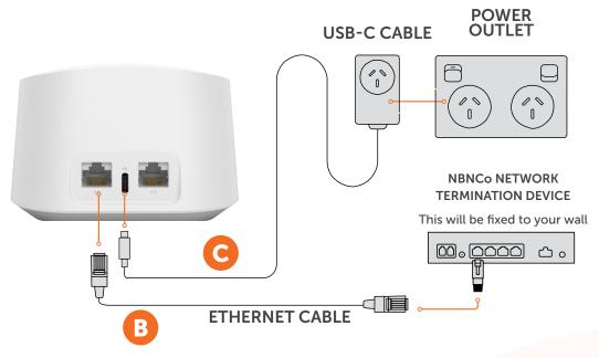
IMPORTANT: You will need to plug the ethernet cable from your eero 6+ into your Network Termination Device's activated Uni-D port. If you are unsure which port has been activated, check your NBN Ready to Go email from us.
