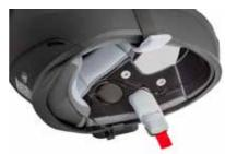
To simplify installation of the speakers into the helmet, first remove the cheek pads and helmet liner. The wires should be installed underneath these linings.
