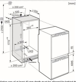
A ventilation gap of at least 40 mm depth must be allowed for behind the appliance for air to circulate. The air inlet to the appliance is via the plinth in the housing unit. The cross-section of the air inlet and outlet must be at least 200 cm<sup>2</sup> to ensure that air can circulate without hindrance.
