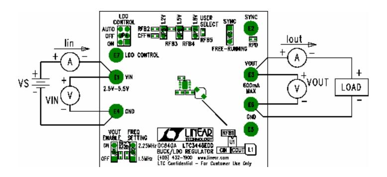
Figure 1. Proper Measurement Equipment Setup
