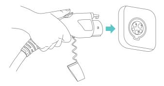
4. Charging begins automatically. Power will be delivered in accordance to the demand of your vehicle. While charging, the Charging Indicator will continuously blink. Always verify your vehicle-charging status by checking the vehicle panel.
