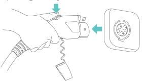
**NOTE:** This charger requires 120 V AC split-phase power supply and is designed to draw a maximum of 12 Amps of continuous current.
