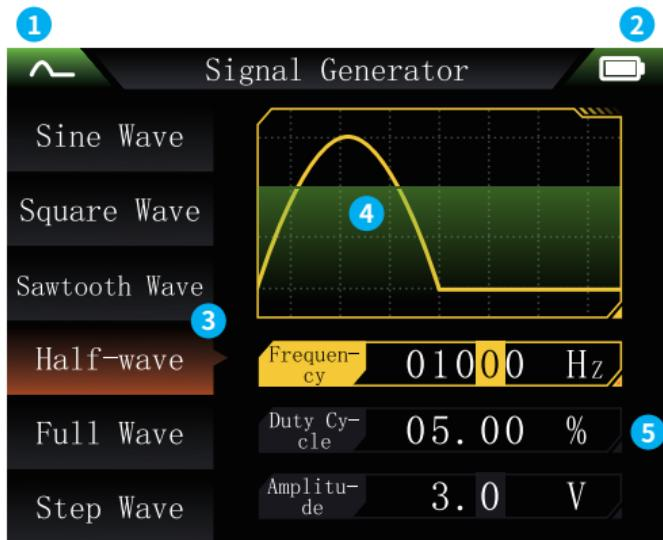
**①Output Status Indication:** a total of 13 types: Detailed statuses are described in section 1.2.
