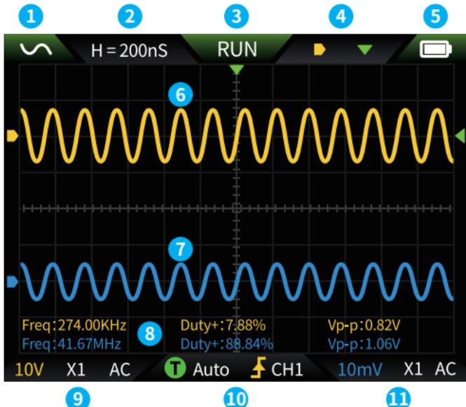
① **Function Generator Interface Status Indication:** 13 waveforms: Sine Wave , Square Wave , Sawtooth Wave , Half Wave , Full Wave , Step Wave , Reverse Step Wave , Index Up , Index Decrease , Direct Current , Multi-audio , Sink Pulse , Lorentz Wave . Gray indicates the waveform output is off.
