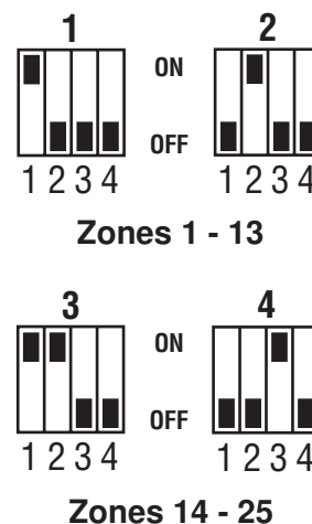
Figure 3.8 2500-RA/RADVR Address Switch Settings
