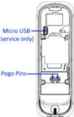
Doorbell Unit (inside view) —
