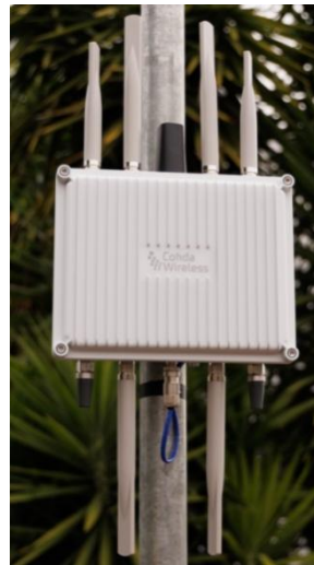
RSU attached to Vertical pole.
