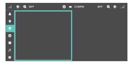
4) Under Split screen mode, you can also press Left / Right Button -> OK Button to select one camera (Camera 1 or 2) you want to view or zoom in. Press the O Button to return to Split screen mode.
