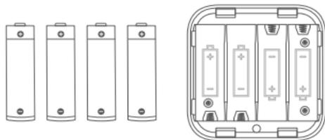
This camera supports both dry battery and rechargeable battery. With 4 batteries of 2400mAh, the camera is able to run about 12 months(Data from HeimVision Lab). However, too high or low temperature, battery quality or other factors will influence the actual running time.
