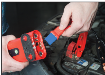
Once it Starts, Disconnect Clamps from Weego 66
