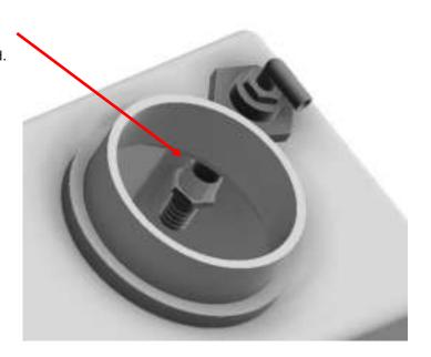
**STEP 2:** Drop the agitator assembly down through the lid opening & connect it to the fitting.
