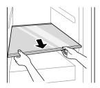
2 Tilt the shelf slightly and remove it by pulling it out.
