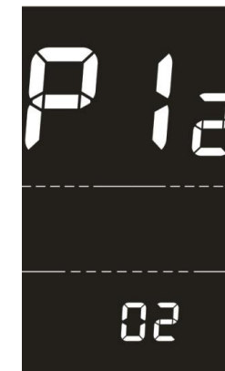
Power boost startup strength setting interface
