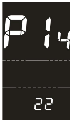
Current-limiting setting interface of the controller
