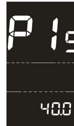
Battery undervoltage value setting interface
