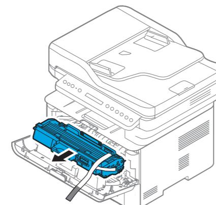
**EN I** Remove the label and the protective cap completely.
