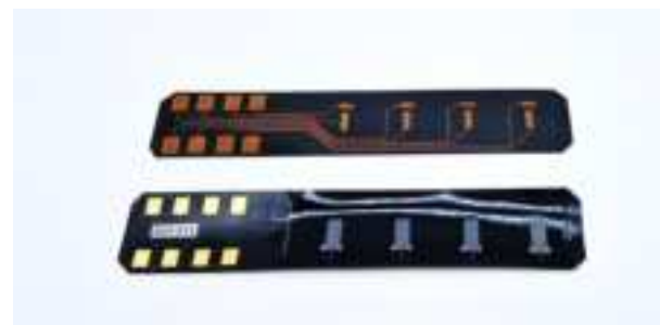
Figure 12 : Example of the integration of several piezoelectric elements manufactured by Wormsensing on a flexible PCB, to obtain a flexible sensor array.
