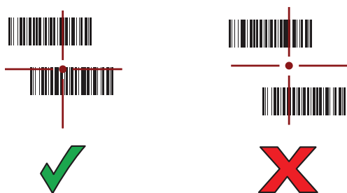
Figure 67 Imager Pick List Mode with Multiple Bar Codes - Extended Range
